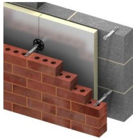
Ancon Two-Part Tie - 2D Detail
